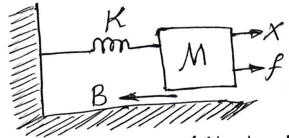
$$M \frac{d^2x}{dt^2} + B \frac{dx}{dt} + Kx = f \quad (**) \text{ By D'Alembert's principle}$$
