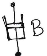
where  $B$  is the damping coefficient. This element is called as dash pot or
